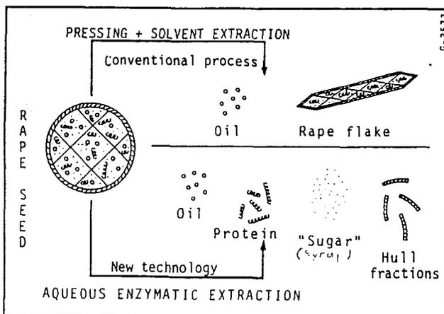
**Fig. 5.1.** Fractions obtained by the enzymatic procedure and the traditional procedure (Olsen, 1988).
